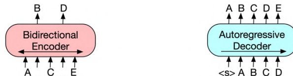
(a) BERT: Random tokens are replaced with masks, and the document is encoded bidirectionally. Missing tokens are predicted independently, so BERT cannot easily be used for generation.
